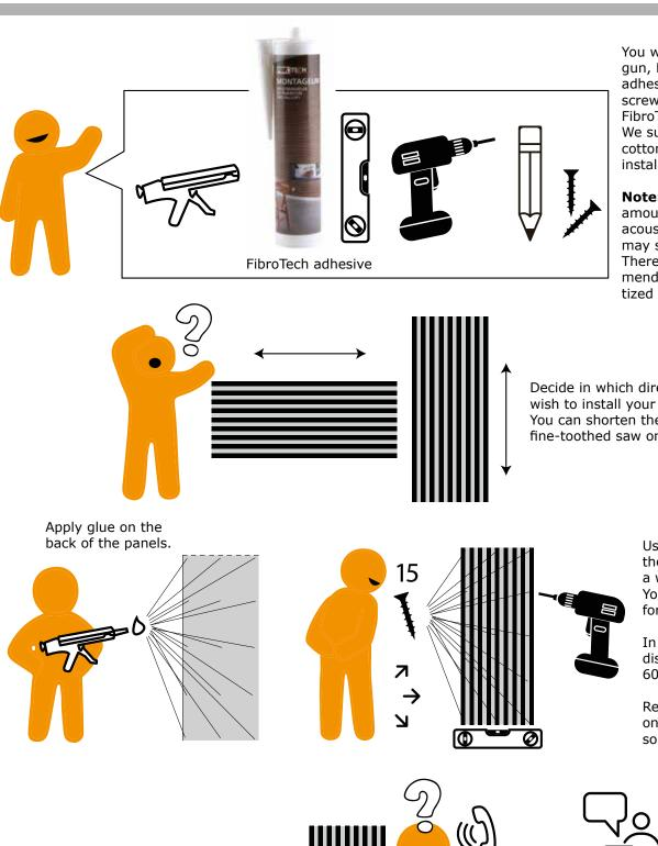
You will need a glue gun, FibroTech assembly adhesive, a spirit level, screwdriver, pencil and FibroTech black screws. We suggest you use cotton gloves when installing your product.
