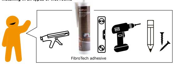
You will need a glue gun, FibroTech assembly adhesive, a spirit level, screwdriver, pencil and FibroTech black screws. We suggest you use cotton gloves when installing your product.
