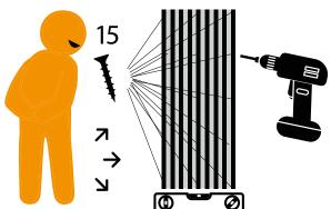
Use screws to install the acoustic panels on a wall or ceiling. You need 15 screws for each panel.
