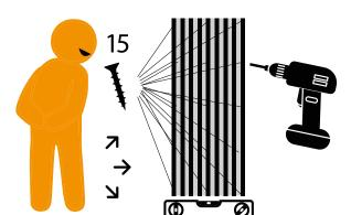
Use screws to install the acoustic panels on a wall or ceiling. You need 15 screws for each panel.
