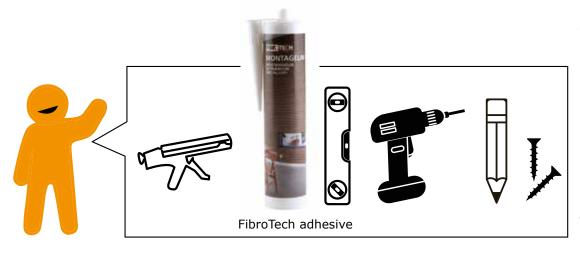
You will need a glue gun, FibroTech assembly adhesive, a spirit level, screwdriver, pencil and FibroTech black screws. We suggest you use cotton gloves when installing your product.
